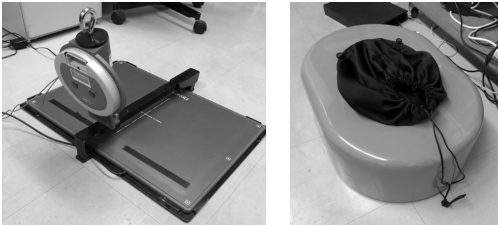
Figure.1. Dynamometer for back strength combined with plantar pressure mat (left) and three-dimensional foot scanner(right).
