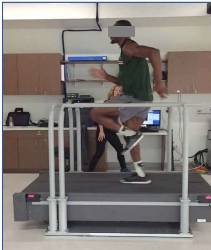
Figure 1. Subject completing 5s run at 6.5 m/s on the instrumented treadmill.
