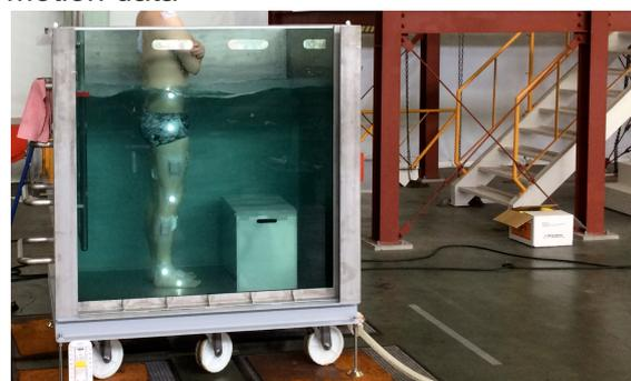
**Figure 2: The made-to-order water tank and 40-cm steel box used as a step**
