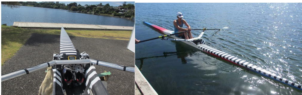
Figure 1: Example of visually textured surface on a rowing boat to better detect water flow.
