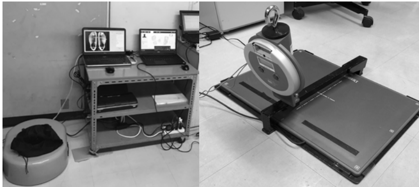
Figure 1. Photo of current measuring system. Foot 3D scanner (left panel) and foot pressure mat combined with strength measurement device (right panel).
