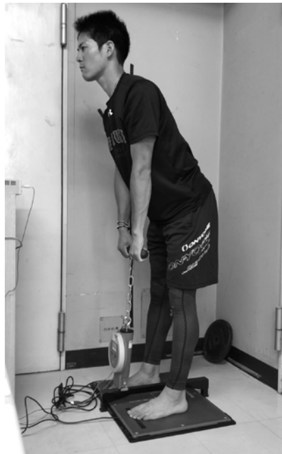
Figure 4. Photo illustrating the testing apparatus when the back strength and underneath foot pressure were measured simultaneously.
