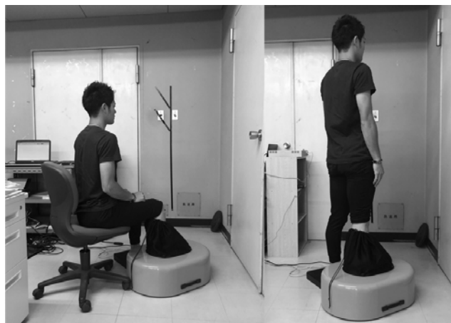
Figure 2. Two postures used to measure foot 3D shape.
